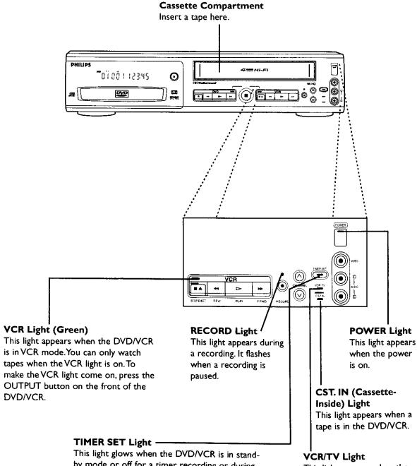
by mode or off for a timer recording or during a One-Touch Recording. It flashes if the TIMER SET button is pressed for a timer recording, but there is no tape in the DVD/VCR. It flashes when all timer recordings or One-Touch Recordings are finished.
